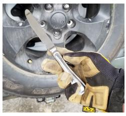
Use a small screwdriver or even a butter knife to remove the center cap from the wheel.
