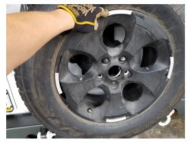
Install 4 pieces of weatherstripping on opposites sides of the wheel face. These are used to help hold the Wheel Shield in place and
