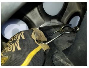
Secure the bungee hooks to one another on top of the spare tire carrier's center support as show in this photo.
